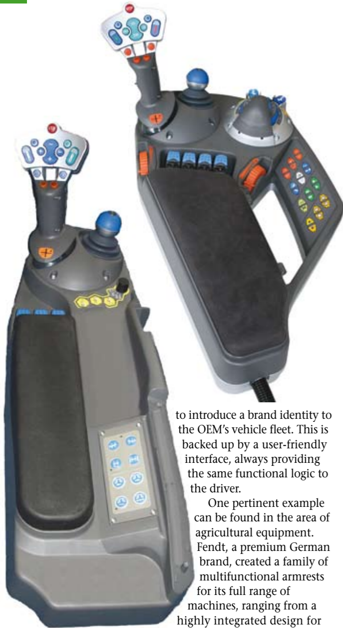
Fendt modular armrest assembly for large (top) and small (above) agricultural tractor applications
